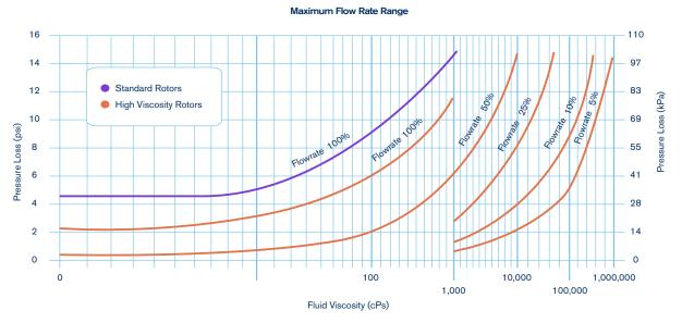
Figure 7: Impact of viscosity on pressure loss for a range of flow rates
