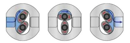
A key distinction of positive displacement flow meters is that they offer direct measurement of the volumetric flow rate. Positive displacement flow meters are frequently specified as they offer high accuracy and repeatability. They readily provide measurement accuracy within +/-0.5% of the true value.
