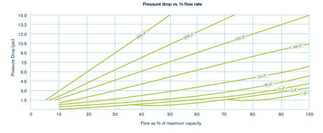
Note: For viscosities greater than 1000 cPs High Viscosity rotors are required
