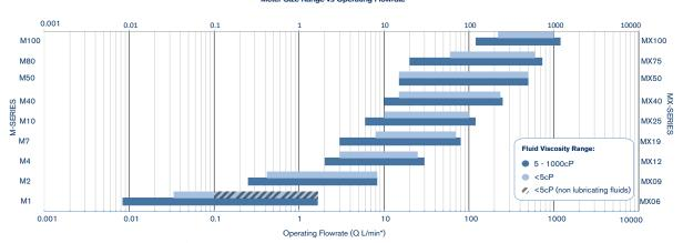
Figure 3: Macnaught Positive Displacement Flow Meters flow rate range selection chart Meter Size Range vs Operating Flowrate
